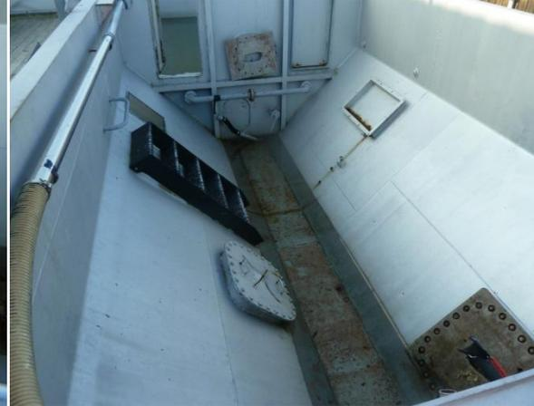
This tank is a simple and practical tool used at the centre for teaching trainees in how to deal with leaks and water intake
